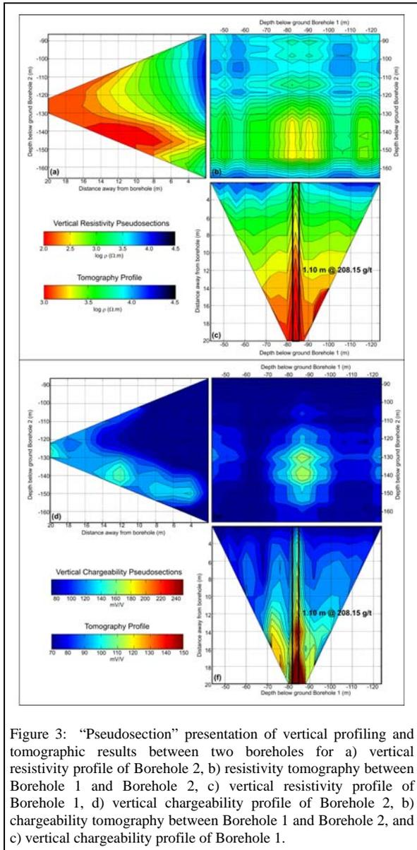
Figure 3: “Pseudosection” presentation of vertical profiling and tomographic results between two boreholes for a) vertical resistivity profile of Borehole 2, b) resistivity tomography between Borehole 1 and Borehole 2, c) vertical resistivity profile of Borehole 1, d) vertical chargeability profile of Borehole 2, e) chargeability tomography between Borehole 1 and Borehole 2, and c) vertical chargeability profile of Borehole 1.
