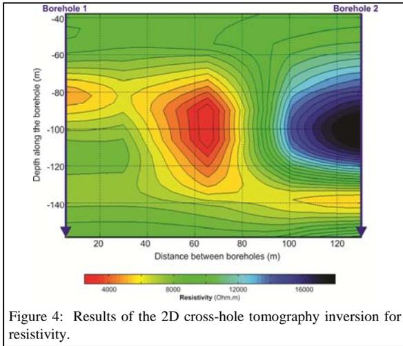
Figure 4: Results of the 2D cross-hole tomography inversion for resistivity.
