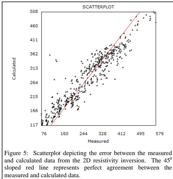
Figure 5: Scatterplot depicting the error between the measured and calculated data from the 2D resistivity inversion. The 45° sloped red line represents perfect agreement between the measured and calculated data.
