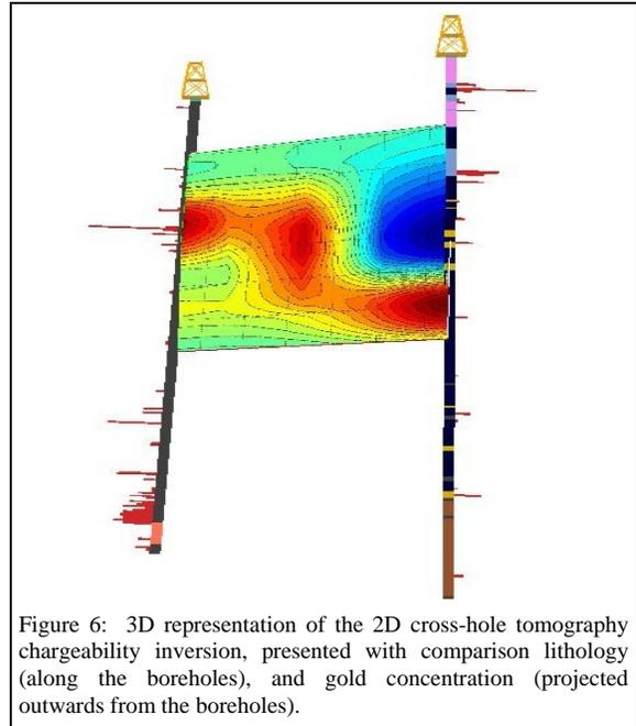
Figure 6: 3D representation of the 2D cross-hole tomography chargeability inversion, presented with comparison lithology (along the boreholes), and gold concentration (projected outwards from the boreholes).
